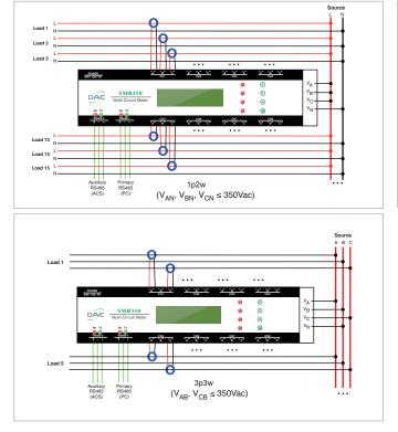
Wiring Diagram Note: The number of CTs that can be used is not limited to what is shown in these diagrams
